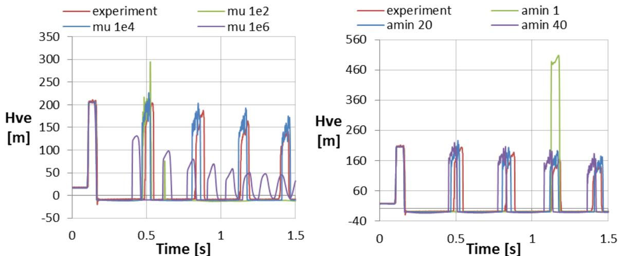
**Fig. 12** Comparison simulation results obtained with SIMSEN free-gas mixture model and MOC-DGCM model with experimental at the downstream valve for results for  $C_0=0.3$  m/s (left) and for  $C_0=1.4\text{m/s}$  (right) over 1.5s
