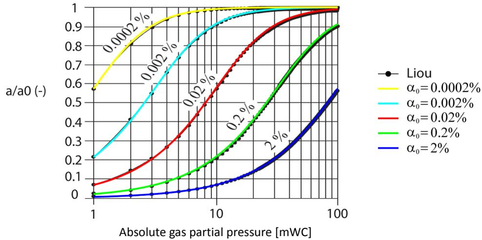
**Fig. 4** Wave speed ratio as function of the initial void fraction  $\alpha_0$  and of the absolute gas partial pressure ( $h-Z-Hv$ ) (adapted from Liou [6])
