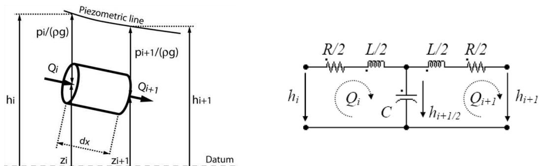
Fig. 1 Equivalent scheme of a pipe
