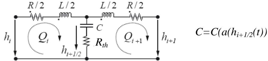
Fig. 7 Equivalent scheme of an elementary pipe with water column separation including pressure dependency of the wave speed and thermodynamic damping
