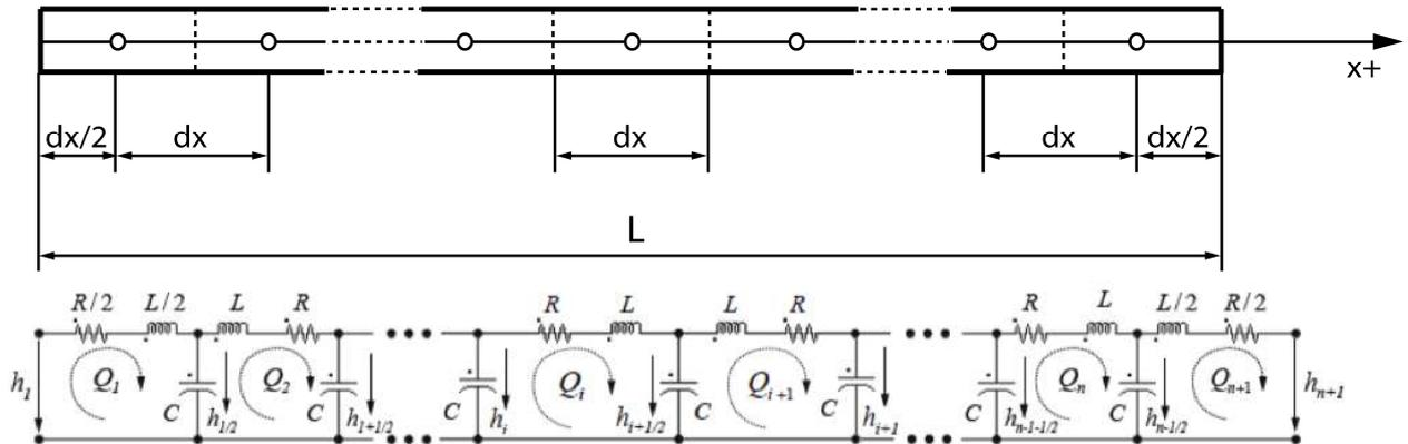
Fig. 2 Equivalent scheme of a whole pipe discretized in “ $n$ ” elements
