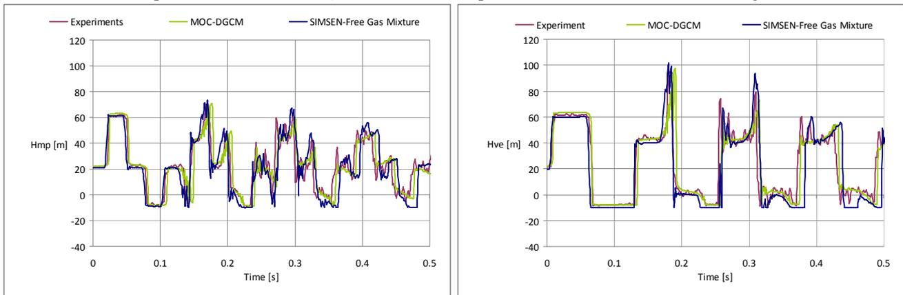
**Fig. 10** Comparison simulation results obtained with SIMSEN free-gas mixture model and MOC-DGCM model with experimental results for  $C_0=0.3$  m/s at the midpoint (left) and downstream valve (right)
