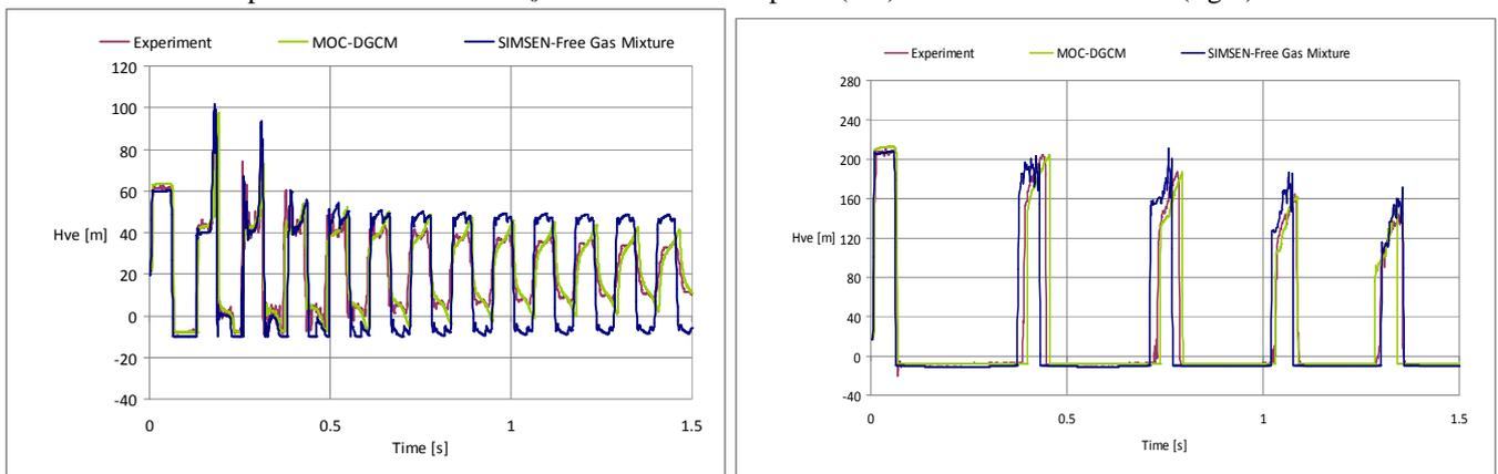
**Fig. 11** Comparison simulation results obtained with SIMSEN free-gas mixture model and MOC-DGCM model with experimental at the downstream valve for results for  $C_0=0.3$  m/s (left) and for  $C_0=1.4$  m/s (right) over 1.5s
