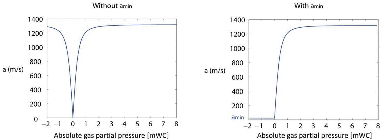
**Fig. 5** Wave speed computed for  $\alpha_0=10^{-7}$  without limitation (left) and with limitation for negative pressure (right)
