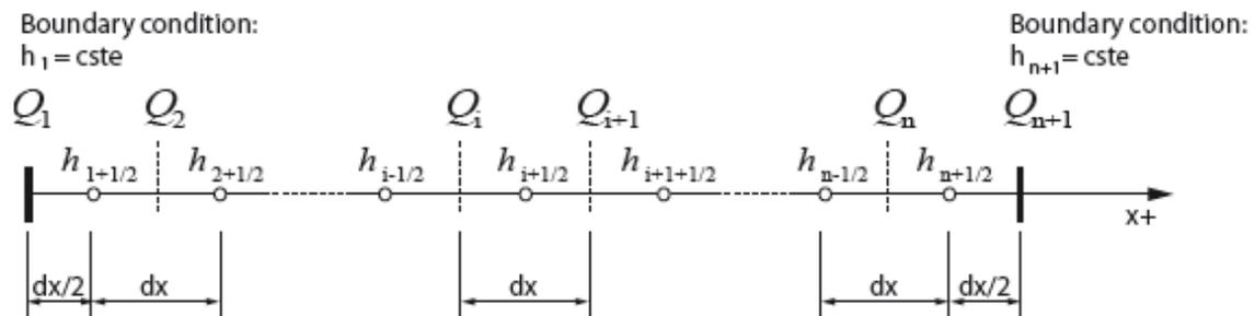
Fig. 3 Spatial distribution of state variables of the pipe model, i.e. discharges  $Q$  and piezometric heads  $h$
