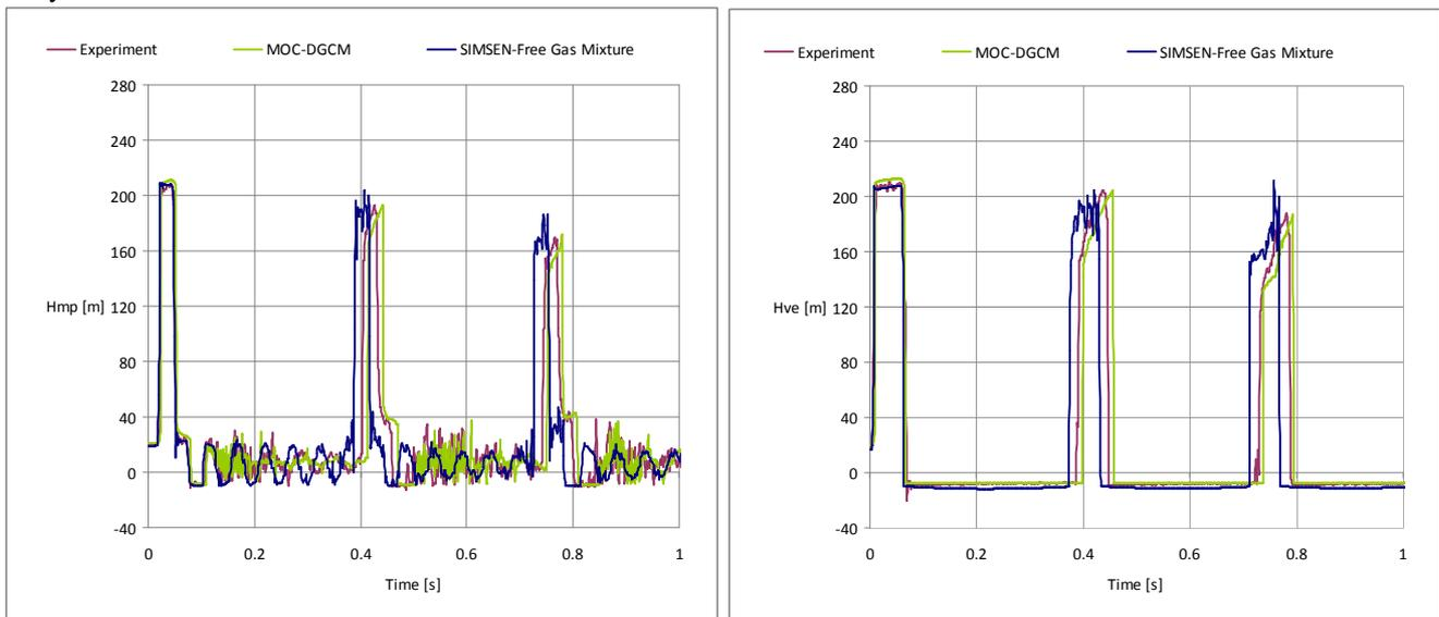
**Fig. 9** Comparison simulation results obtained with SIMSEN free-gas mixture model and MOC-DGCM model with experimental results for  $C_0=1.4$  m/s at the midpoint (left) and downstream valve (right)
