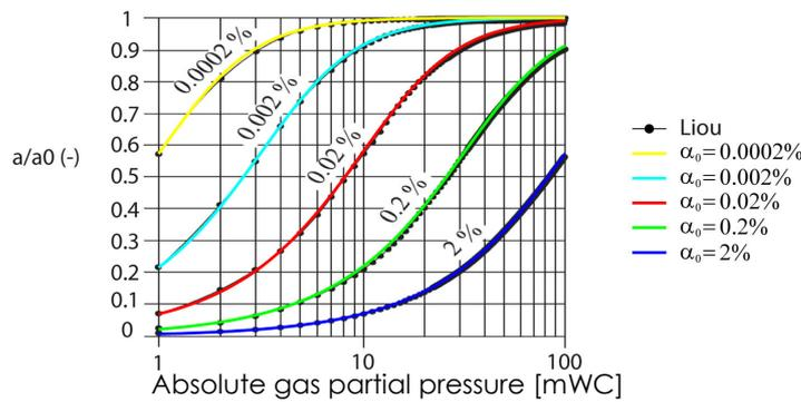
**Fig. 3** Wave speed ratio as function of the initial void fraction  $\alpha_o$  and of the absolute gas partial pressure ( $h-Z-Hv$ ) (adapted from Liou [13]).
