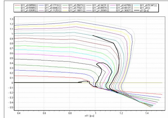
**Fig. 10** Pump-turbine transient operating point in case of emergency shutdown in generating mode in the N11-Q11 plain.
