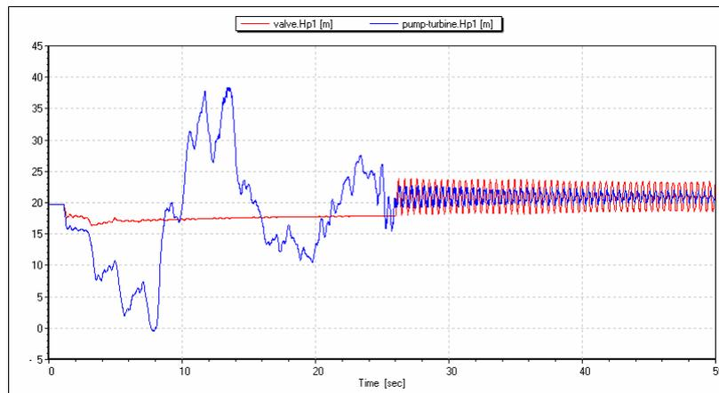
Fig. 13 Comparison of the time evolution of the pressure at the inlet of the draft tube obtained with the pump-turbine and with the valve.
