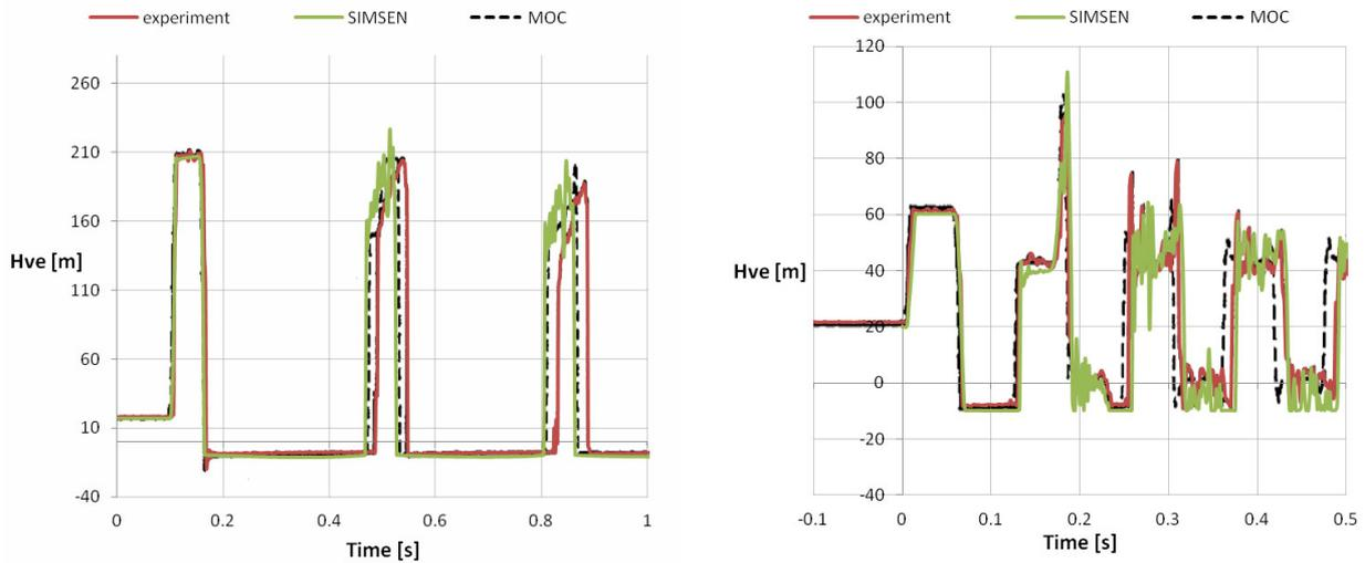
Fig. 6 Comparison simulation results obtained with SIMSEN free-gas mixture model and MOC-DGCM [20] model with experimental results at the downstream valve for  $C_0=1.4$  m/s (left) and for  $C_0=0.3$  m/s (right), see [16]
