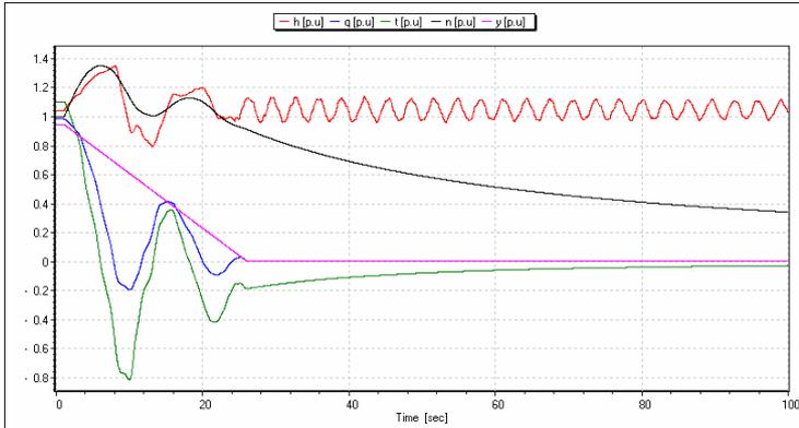
**Fig. 9** Pump-turbine transient behaviour in case of emergency shutdown in generating mode with  $h$  the net head,  $q$  the discharge,  $t$  the torque,  $n$  the rotational speed and  $y$  the guide vane opening all related to rated values.
