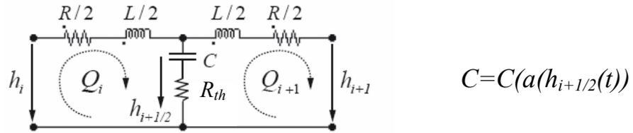
Fig. 4 Equivalent scheme of an elementary pipe with water column separation including pressure dependency of the wave speed and thermodynamic damping.
