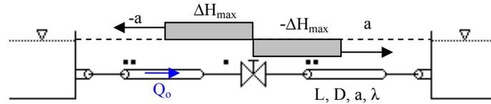
Fig. 7 Water hammer induced by fast ( $T_c < 2L/a$ ) valve closure between two pipes of same size.
