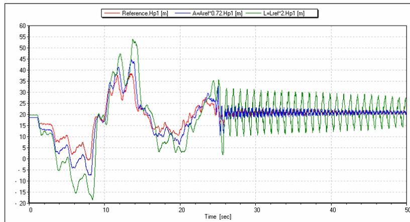
**Fig. 14** Time evolution of the pressure at the inlet of the draft tube obtained with the pump-turbine in case of emergency shutdown in generating mode in case (i) the tailrace tunnel cross section is reduced to 72% of the original cross section and in case (ii) the length of the tailrace tunnel is doubled.
