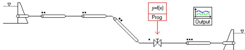
**Fig. 11** SIMSEN model of same case study as Fig. 8 with a valve instead of the pump-turbine.
