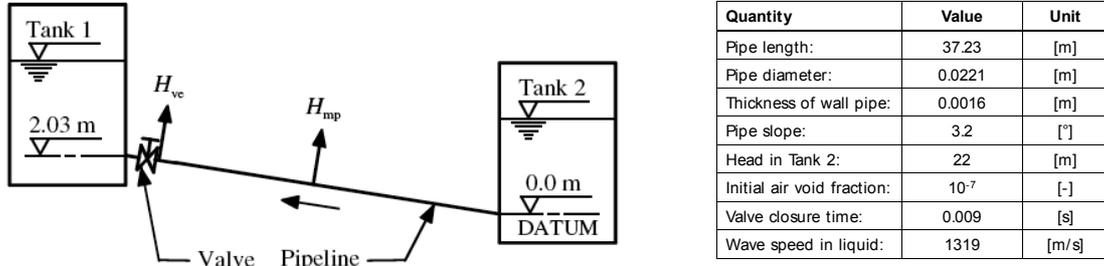
Fig. 5 Test case experimental apparatus, from [19].
