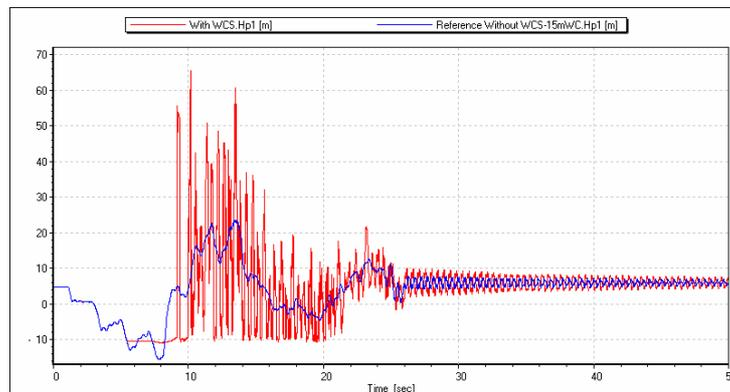
**Fig. 15** Time evolution of the pressure at the inlet of the draft tube obtained with the pump-turbine in case of emergency shutdown in generating mode with and without water column separation model (WCS) if the tailrace water level is reduced by 15m (case A).
