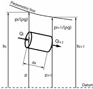
Fig. 1 Elementary hydraulic pipe of length dx.
