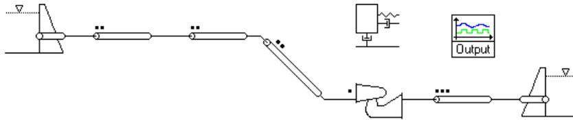
Fig. 8 SIMSEN model of the pump-turbine case study with simplified layout.
