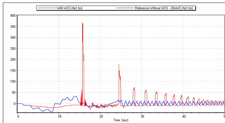
**Fig. 17** Time evolution of the pressure at the inlet of the draft tube obtained with the pump-turbine in case of emergency shutdown in generating mode with and without water column separation model (WCS) if the tailrace water level is reduced by 20m and the length of the tailrace tunnel is doubled (case C).
