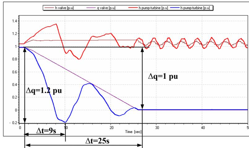
Fig. 12 Comparison of the time evolution of the pump-turbine discharge and net head of the system of Fig. 8 with the discharge and net head of the valve of system of Fig. 11 all related to rated pump-turbine values.
