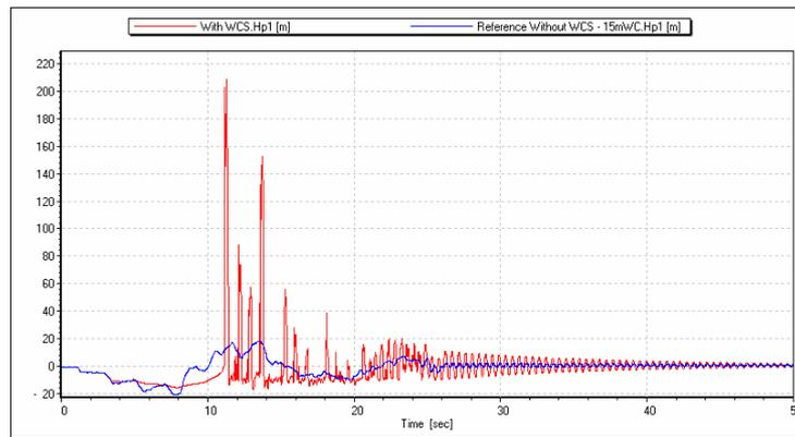
**Fig. 16** Time evolution of the pressure at the inlet of the draft tube obtained with the pump-turbine in case of emergency shutdown in generating mode with and without water column separation model (WCS) if the tailrace water level is reduced by 20m (case B).
