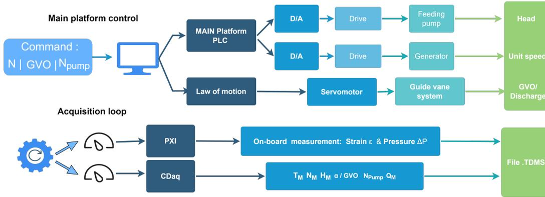
Figure 1: Data flow of the test rig and data acquisition system.
