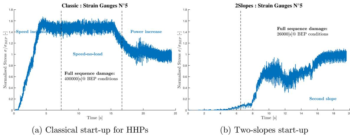
Figure 6: Stress comparison between the two-slopes start-up and the classical sequence.
