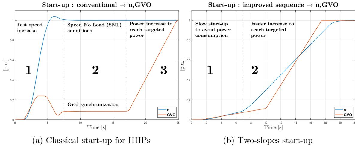
Figure 4: Comparison between two-slopes and classical start-up sequences.
