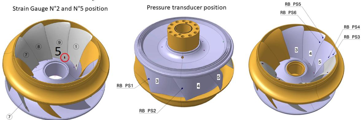
Figure 3: On-board measurements set-up and location of the pressure transducers and strain gauges.
