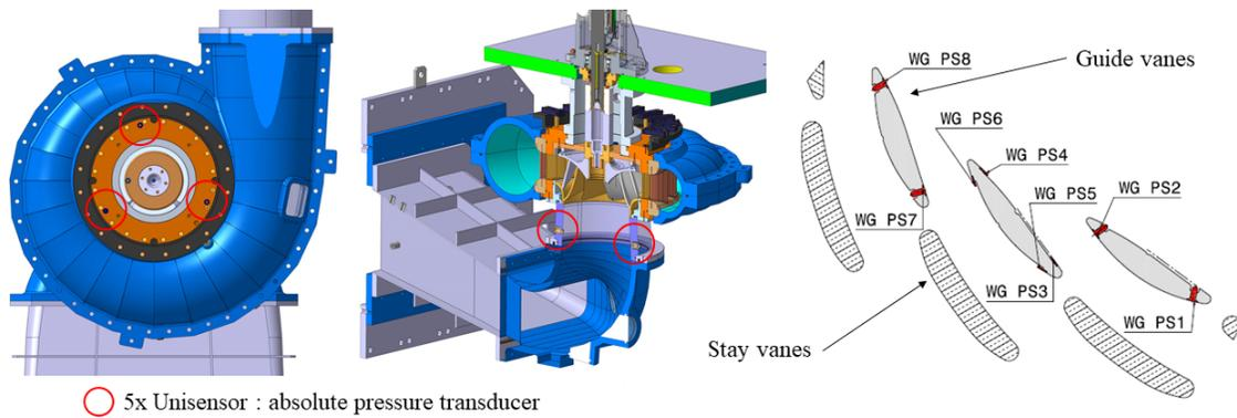
Figure 2: Static frame pressure measurement set-up: positioning of the pressure sensors in the runner's vicinity.
