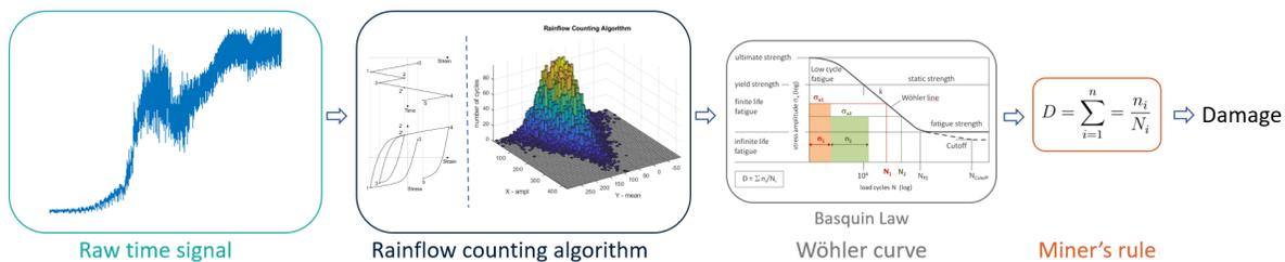
Figure 5: Damage computation methodology.
